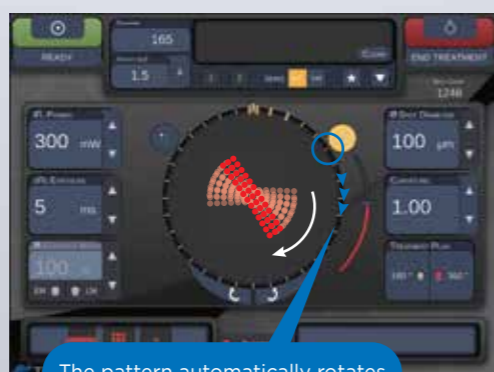
The pattern automatically rotates 11.25 degrees to align adjacent to previous treatment site
